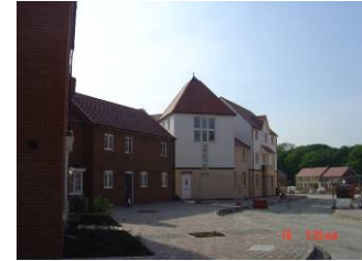
Figure 3: More recent development in Ashford that visually suggests 'Kent'. Continuous frontage creates positive street enclosure leading towards a small square. However, strongly rear serviced layouts such as this can give rise to inappropriate parking and so the place-making role of continuous frontage needs to be properly balanced with streets designed to accommodate unallocated on-street parking.
